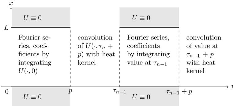
Fig. 1. For an arbitrary number of barrier periods consider the coordinate change (2.3) and solve the boundary value problem by Fourier series within the barrier period and by convolving with the heat kernel when the barriers are not active.
